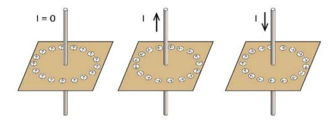
Looking at the first diagram (from the left) ,we see if there is no current flowing in wire , compasses will be aligned along the north-south direction.
